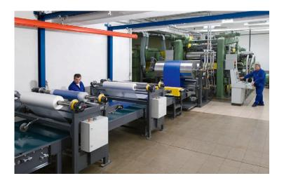
oller coverings must be abrasion-resistant, dissipative, ozone- and temperature-resistant and conductive – preferably all of these at the same time.
